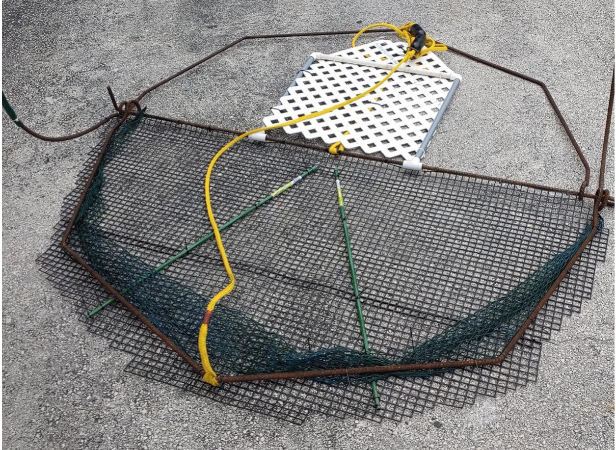
Figure 8. Design 8, Rigid plastic netting will be outside the rebar frame with either bars or an additional frame to prevent it from being able to be inverted through the rebar frame from below.
