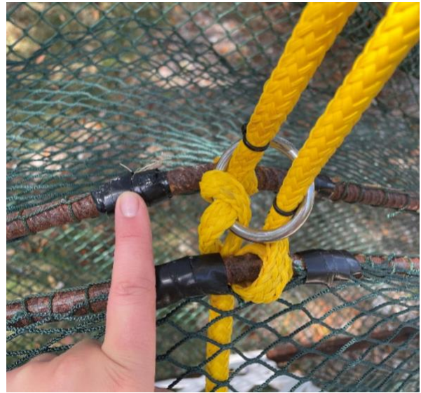
Figure 13. Trap harness with 1-inch ring. Finger used to show distance. Trap is closes tighter with smaller ring.
