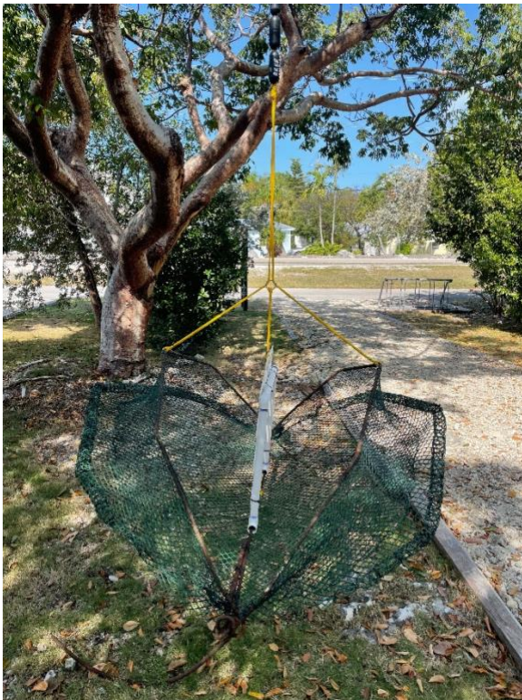
Figure 2. (3) Trap is fully closed and off the ground. Mesh is billowing. Rigid plastic is sitting off trap frame.
