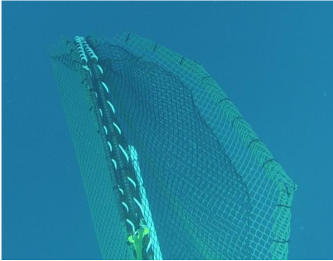
Figure 3. GoPro footage of trap retrieval with “baffle design”. Once closed and being brought up from the bottom, depending on waves and current, one side of the design pushes up against the frame.
