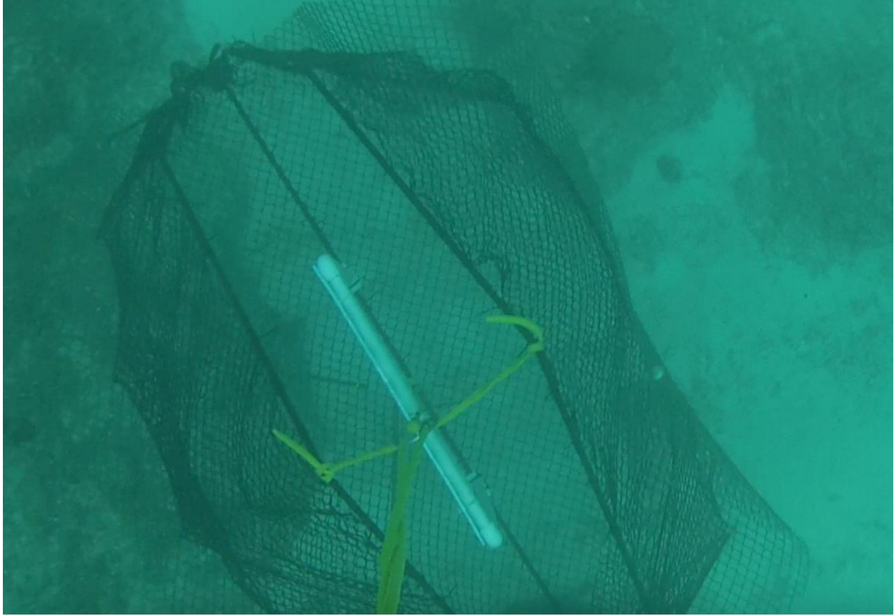
Figure 11. Design 8, The “baffle design” allows for a adequate billowing, and the billow may not be affected by a cross current as much as a frame with soft netting alone.
