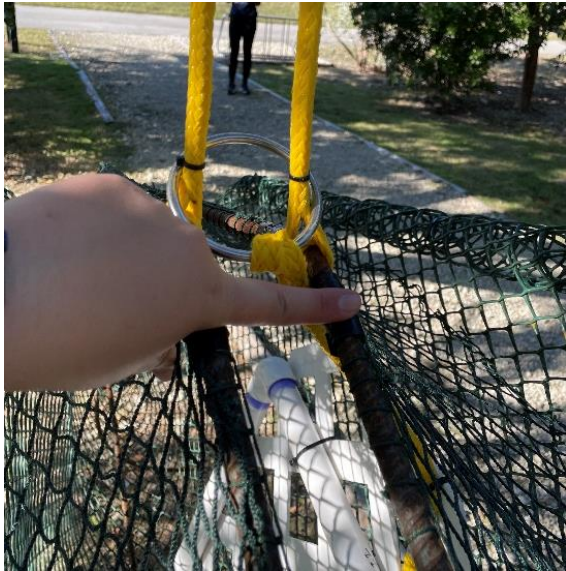
Figure 12. Trap harness with original 3-inch ring. Finger used to show distance between the top frame arms of closed trap.
