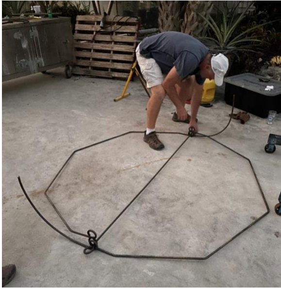
Figure 15. Dr. Steve Gittings of NOAA, checking newly bent lionfish trap frames to make sure hinges are not binding with newly bent axle.
