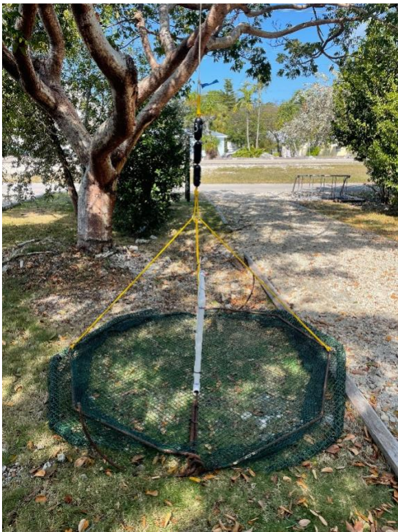
Figure 5. (1) Trap open on the ground. Rigid plastic netting and mesh lay flat on the ground. FAD is taught.
