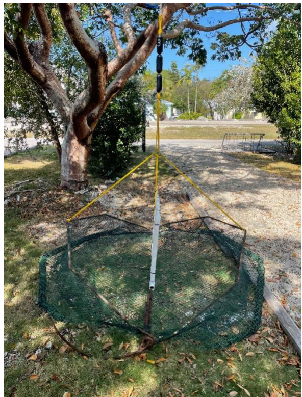
Figure 6. (2) Trap is starting to close. Mesh is pulled up first to create space for billowing. The rigid plastic follows.
