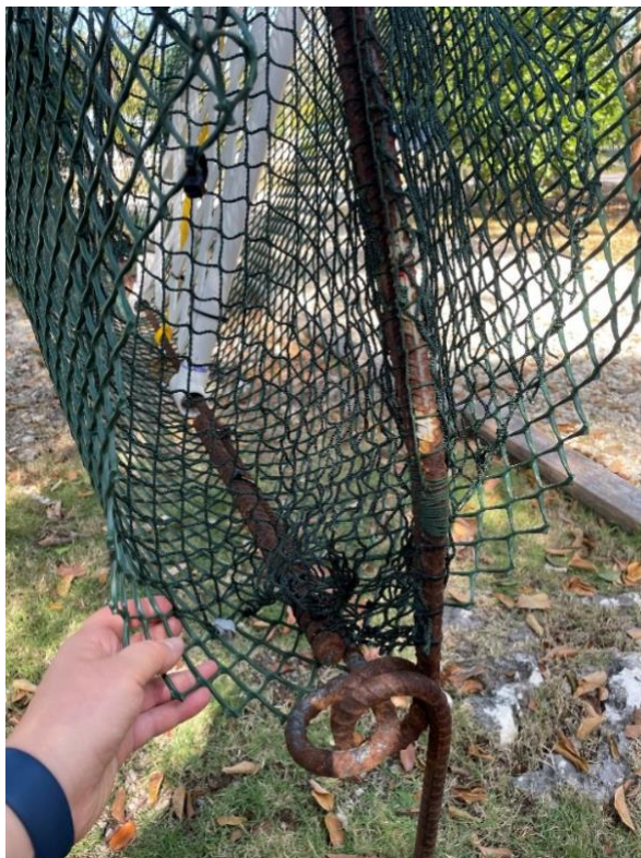
Figure 14. Area of trap near hinges. Zip ties used to close the edges of trap and not impair hinges. Hinges are visibly clear of mesh and rigid plastic netting. Axle eye loop is closed directly around door eye loops to keep doors closed tightly and prevent them from sliding side to side.
