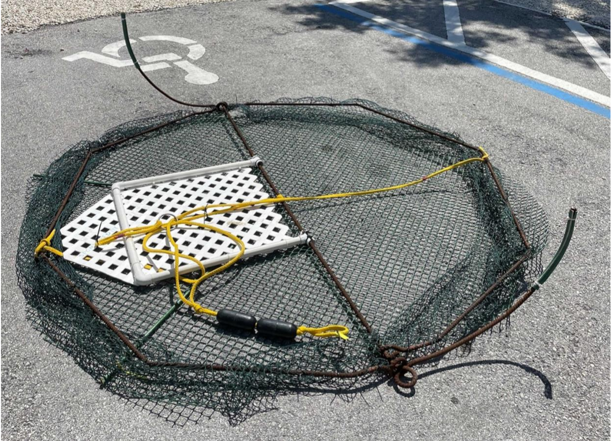
Figure 9. Design 8, Rigid plastic netting will be outside the rebar frame with either bars or an additional frame to prevent it from inverting through the rebar frame from below. The green plastic netting shown here and in the remaining figures is stronger than the black plastic netting in the figure above and will likely be the material of choice.
