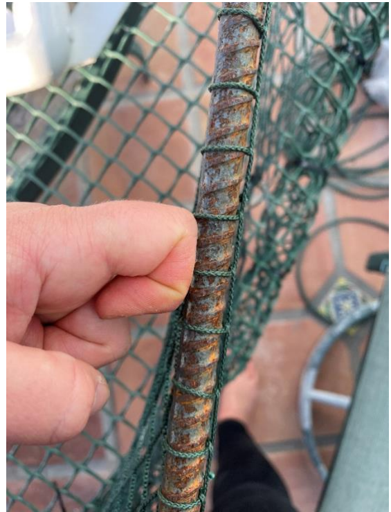
Figure 4. Trap lacing to attach netting to rebar frame and rigid plastic netting is less than an inch apart, closer than previous trap designs. Added drag from the rigid plastic netting was counteracted with closer lacing to increase the surface area being pulled on.
