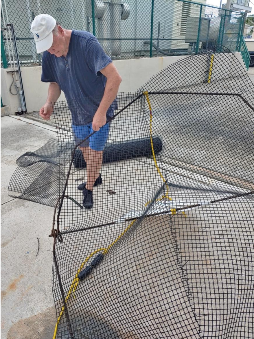
Figure 5. Design 6, Sewn layers of stiff black mesh designed to allow for billow
