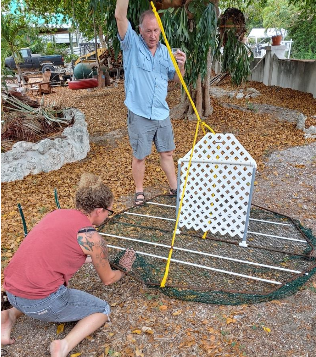
Figure 6. Design 7 Horizontal bars are placed across the netting on the inside to create a ceiling to prevent turtle from getting traps or disorientated by netting. Demonstration that the gaps would need to be narrow enough to prevent small turtles from going between the bars.
