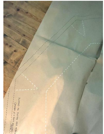
Figure 14 (above) The trap frame is traced in the dotted white line. The dotted white line Vs are where to make the cuts in the hard plastic lattice. The solid black line is 12" above the trap frame and the dotted black line is 14" above the trap frame.
