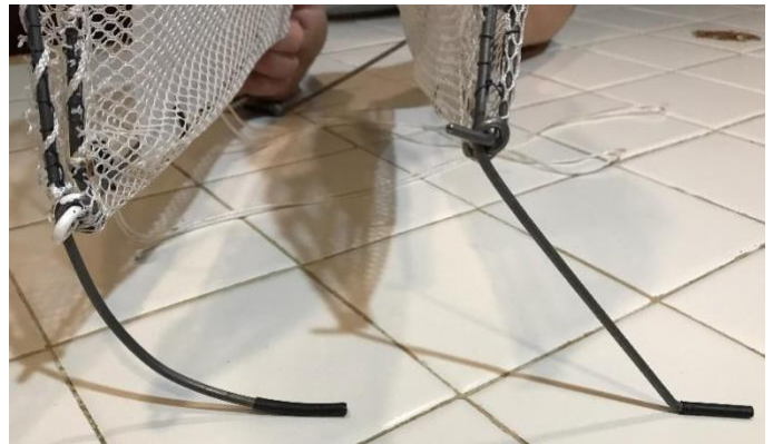
Figure 7. Curved (left) and straight (right) deflectors on 1/6 scale model traps. Black covers on tips simulate hose used to cover end of rebar.
