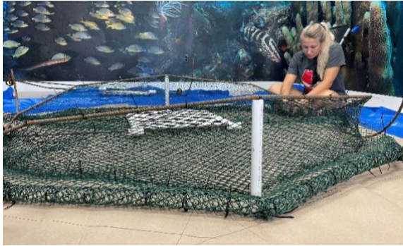
Figure 18. The netting of the trap cut and attached with zip ties before being sewn onto the frame and hard plastic lattice.
