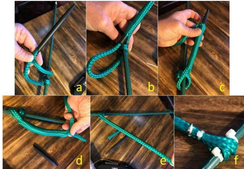
Figure 22. Steps to attach ring line to axle.
