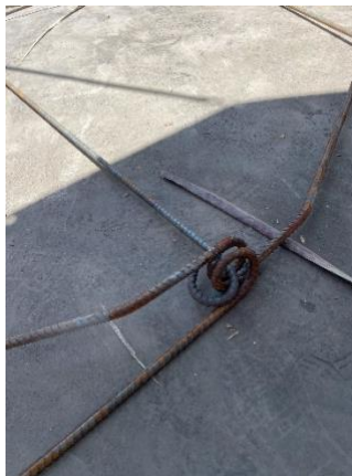
Figure 5 (near right). End loop hinge (left) with axle inserted through it and deflector hinge (right), and loop on the end of axle connecting the two frames.
