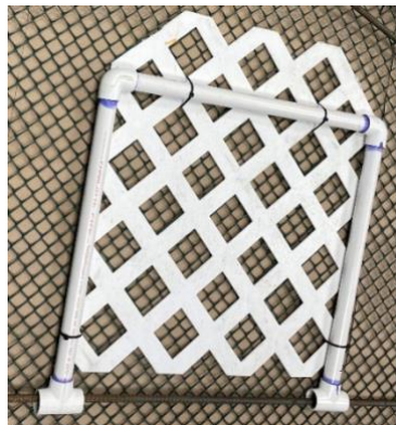
Figure 12. FAD attached to bracket with cable ties without the right line or harness attached. The gap between the axle and FAD can be clearly seen. This allows the FAD to rotate freely and not bind.
