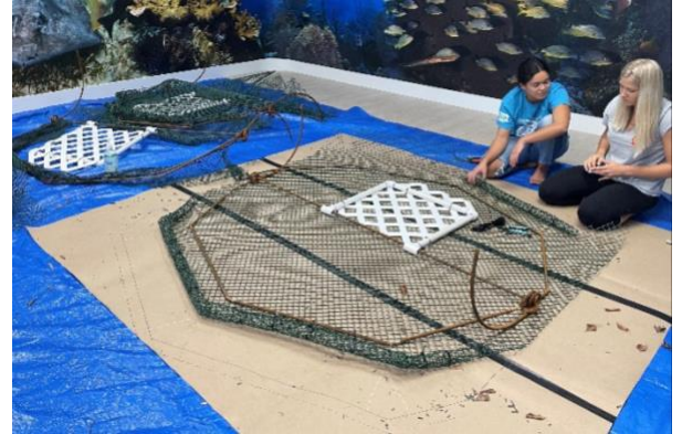
Figure 17. Using fingers to show about a 2" distance between the frame and the rolled plastic lattice.
