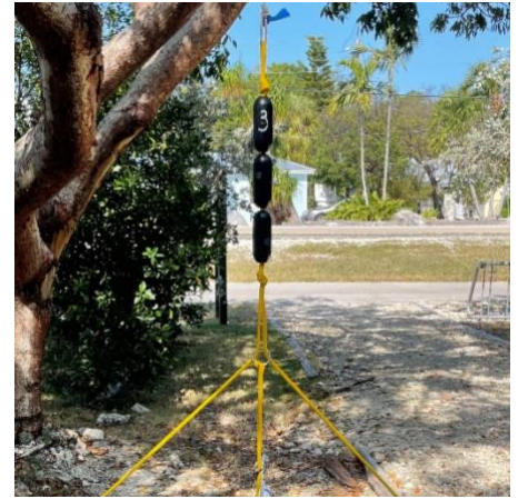
Figure 24. Three 1-3/4"x5" floats below loop at top of bridle, secured with overhand knots above and below the floats.
