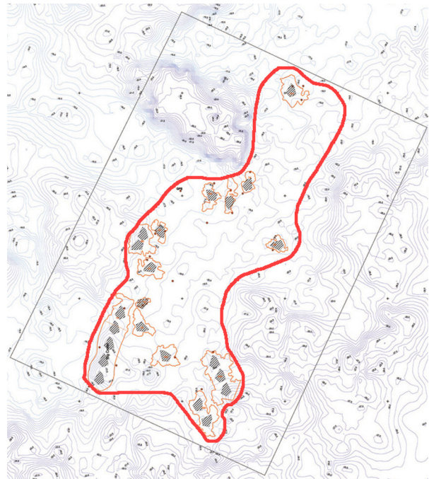
Figure 3. A bathymetric map showing the placement of the restoration modules. The area within the red line denotes the area surveyed; high profile, undamaged areas were avoided.
